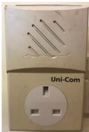
◀ You may have noticed this device plugged into a socket in the downstairs hall – this is a receiver for the bell which is located by the rear entrance door.
